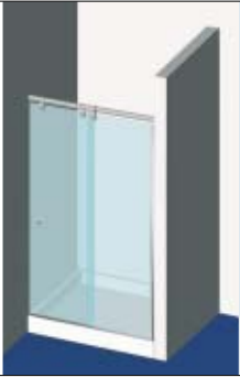
2820.XX.1 CASE 1 - Wall to wall sliding door: A sliding door and a fixed panel. Sliding door on the left or right side. Wall to wall distance: 2200 mm. Maximum door weight: 30 kg.
