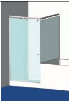
2820.XX.4 CASE 4 - Frontal access sliding door: A sliding door and a fixed panel, a fixed panel and a fixed panel on the bath-tube. Maximum tray width 1100 x 1100 mm. Maximum door width 550 mm. Maximum door weight: 30 kg.
