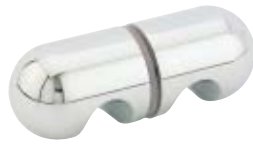
3066 Round head knob 40 mm Ø for 6 to 10 mm thick glass. Fits on 16 mm Ø hole.
